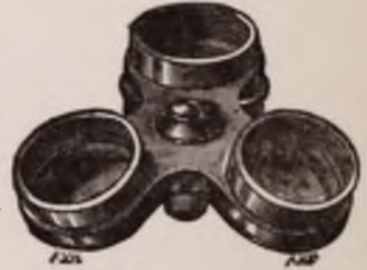
FIG. 21. Triple nose piece or revolver for quickly changing objectives (Queen & Co.).
