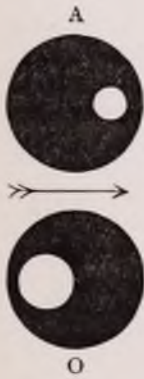
FIG. 49. Very small Globule of Oil (O) and an Air Bubble (A) seen by Oblique Light. The arrow indicates the direction of the light rays.
