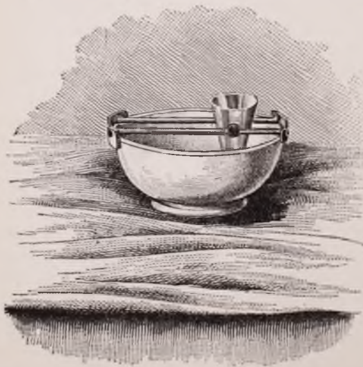
FIG. 81. Waste Bowl (from the Reference Hand Book of the Medical Sciences, Supplement ). "The apparatus is easily constructed and exceedingly useful. The ends of two glass rods of the proper length are fastened into two strips of lead, slightly curved to fit around the margin of an ordinary bowl. Between the glass rods is a tin funnel, held in position by flanges of tin which may be bent around the rods and permit the funnel to slide back and forth. The rods are a convenient resting place for the slide while in process of preparation.
