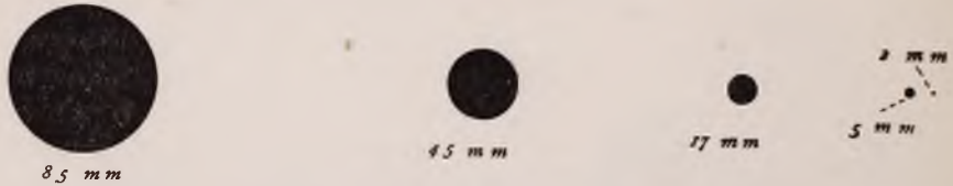
Fig. 23. Figures showing approximately the actual size of the field with objectives of 85 mm., 45 mm., 17 mm., 5 mm., and 2 mm., equivalent focus, and ocular of 37½ mm., equivalent focus in each case. This figure shows graphically what is also very clearly indicated in the table (§ 37).
