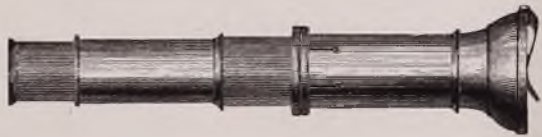
Small hand microscope, convenient for sea side p. 177
