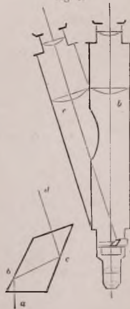
Binocular microscope as recently arranged by Mr. Wenham, and now generally adopted. p. 14.
