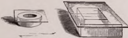
To illustrate the manner in which thin glass may be perforated for making thin glass cells p. 73.
