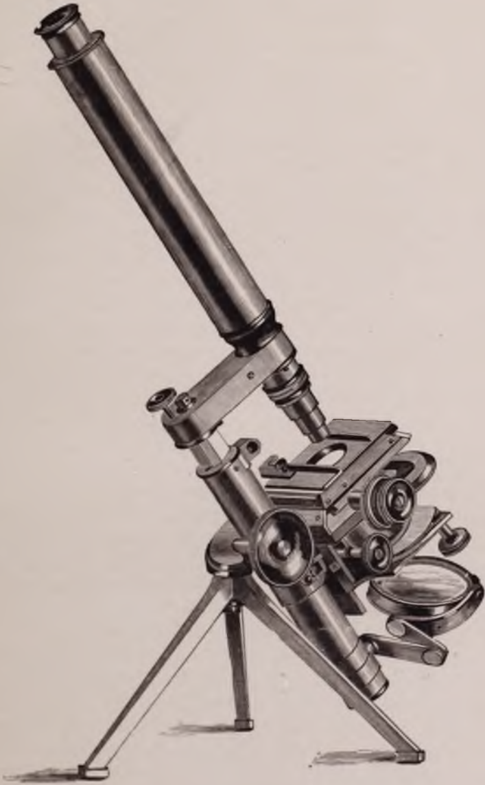
Folding microscope of Messrs. Towell and Lealand, adapted for all purposes. This instrument may be used for the highest powers. It is perfectly steady, and is packed with all the required apparatus and instruments in a case 12 inches long, 7 inches wide and 3 inches deep. p. 10.
