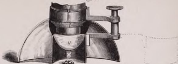
Parabolic reflector of Mr. Beck, with Mr. Sorby's flat mirror, M. p. 237.
