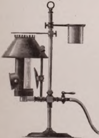
Gas microscope lamp, with water bath, &c arranged by Mr. Highley. p. 25.
