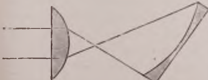
Arrangement for obtaining parallel rays as recommended by Gerlach p. 308.
