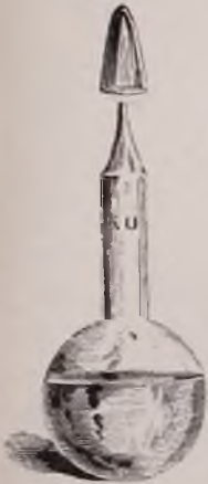
Bulb with capillary orifice for testing small quantities of matter. p. 261.
