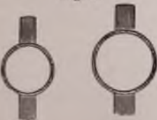
Flat brass rings, for cutting circles of thin glass. p. 71.
