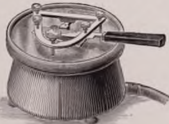
Freezing microtome, as suggested by Mr. Williams of the Quekett Club, and made by Swift. p. 91.
