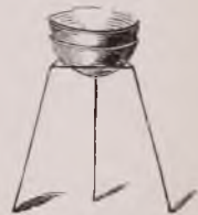
Porcelain basin arranged for a water bath. p. 50.
