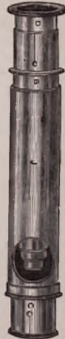
Waistcoat pocket microscope, only 4 inches long. Made by Mr. Hignley. p. 20.
