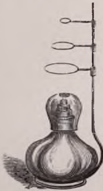
Spirit lamp, with wire stand attached for supporting watch-glasses &c. p. 49.
