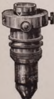
New centring nose-piece, designed by Mr. Swift. p. 9.
