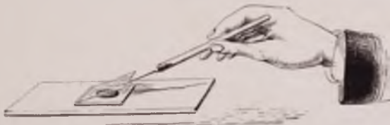
To illustrate the manner in which the thin glass is allowed to fall gradually upon an object mounted in fluid. p. 82.
