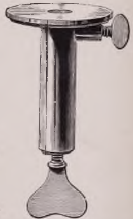
Instrument for cutting thin sections of wood, &c. p. 89.
