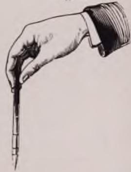
Writing diamond, for cutting thin glass. pp. 63, 70.
