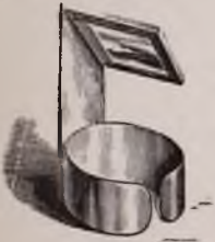
Neutral-tint glass reflector for drawing p. 33
