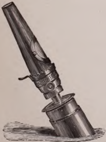
Round-tipped lamp, with shoe. Showing position when used for examining objects with direct light. p. 25.
