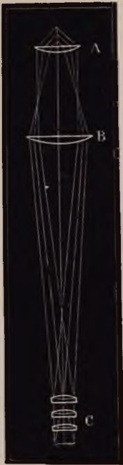
Diagram of compound microscope. p. 3
