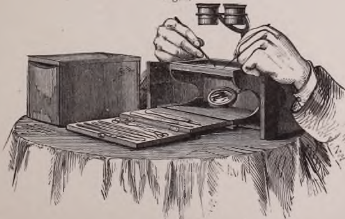
Dr. Lawson's binocular dissecting microscope, made by Collins. On the left, the instrument is shown folded up. p. 21.
