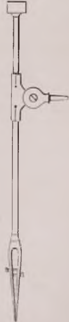
Forceps which can be attached to the stage of the microscope for holding objects during examination, with low powers p. 52
