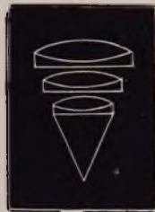
Compound glasses of an achromatic object glass. p. 8.
