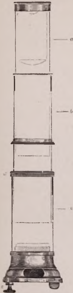
Pocket or clinical microscope. Half the real size p. 18.
