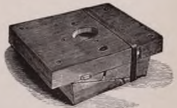
Professor Quekett's dissecting microscope. The instrument folded up for travelling p. 21
