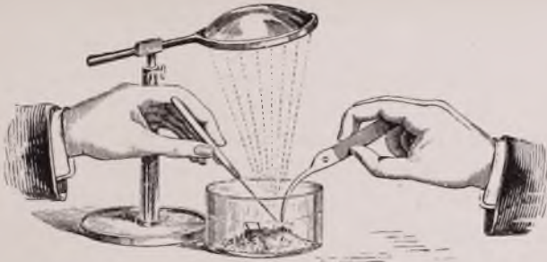
Arrangement for making minute dissections under water. p. 91.
