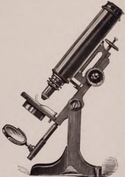
New histological microscope, arranged by Mr. Collins. The fine adjustment is according to a new plan, and is very simple and efficient. pp. 11, 13.
